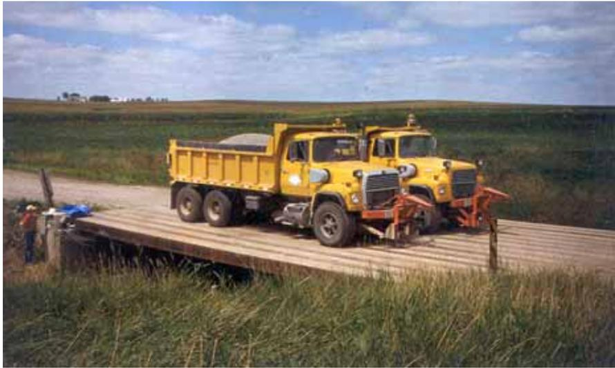
Figure 1.2. Field testing of the original Beam-in-Slab Bridge System.
